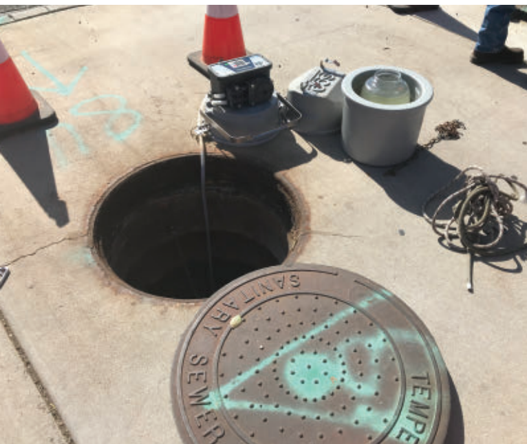
A small automated machine perches at the edge of a maintenance hole, ready to retrieve wastewater samples (like the one in the gray container) from the Tempe, Ariz., sewage system.
